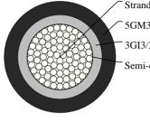
Stranded Tinned Copper Conductor 5GM3/HM3 Rubber Outer Sheath 3GI3/3GJ3 Rubber Insulation Semi-conducting Layer
